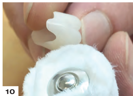
Smooth out attachment point with fine-grain diamond burs. Final polish using cotton/linen buffs.
