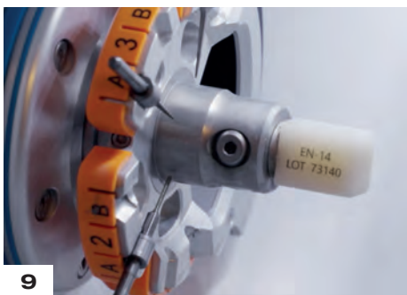
Milling of the Block to make the final crown.
