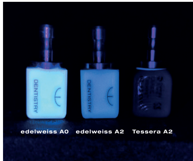
edelweiss CAD/CAM BLOCKS show better fluorescence than a ceramic CAD/CAM block
